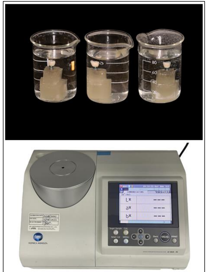
Figure 3: Sample immersed in distilled water and colour analysis done using spectrophotometer (Konica Minolta CM5)
