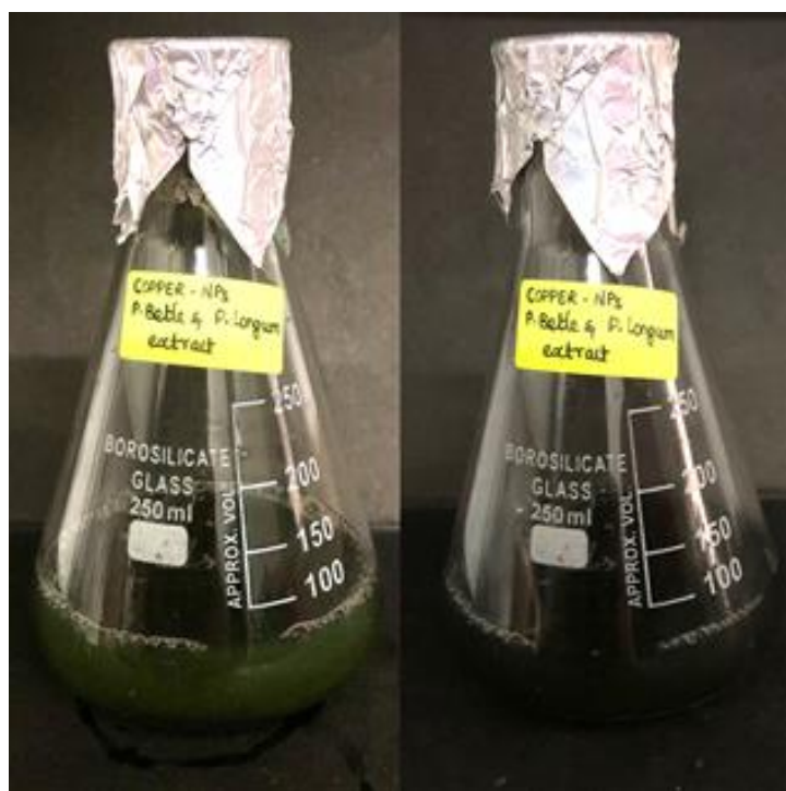
Figure 3: Shows a color shift from dark green to black, demonstrating the formation of copper nanoparticles.
