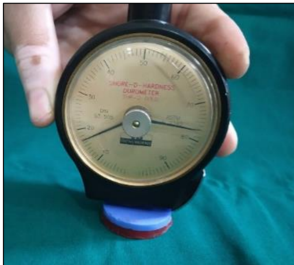
Figure 4: Shore D hardness measuring device for measuring surface hardness for sample
