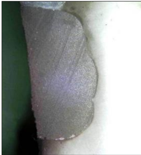
Figure 1: No dye penetration (Score 0)
