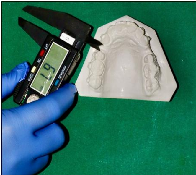
Figure 2: Measurement of tooth movement with digital vernier calliper
