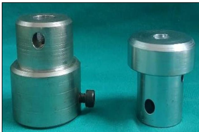
Figure 2a: Customised jig parts
