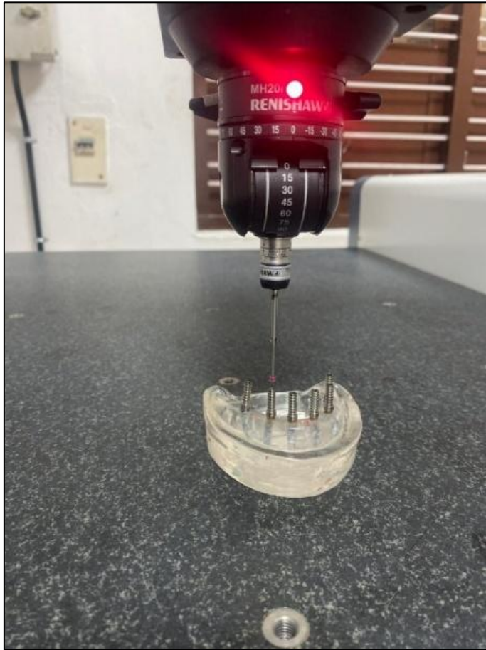
Figure 6: Coordinates measured using coordinate measuring machine
