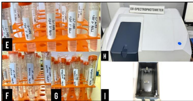
Figure 2: (E) (F) (G) Cement pellets immersed in distilled water (H) UV Spectrophotometer (I) Analysis in UV Spectrophotometer.
