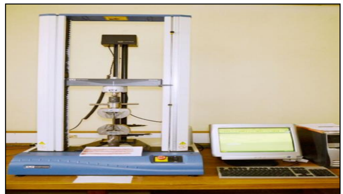
Figure 2: Universal mechanical testing machine (Instron, Model 3366, USA)
